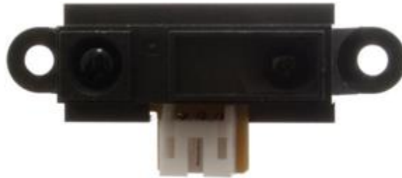
Figure 23 - Shows an image of the Infrared sensor designed by Sharp that we will be implementing in our table. Courtesy of Oomlout, Creative Commons 2.0
