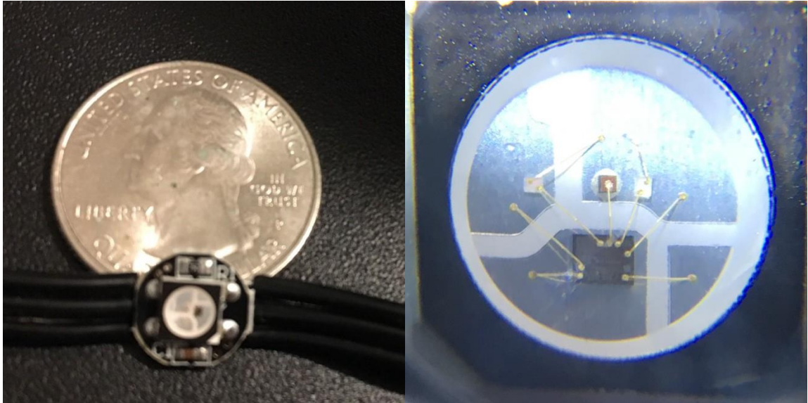
Figure 14 - Illustrates compact nature of WS2812-B versus a 60x magnification of same WS2812-B. Created by Mikey Garrity
